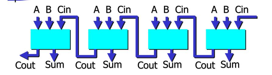
The carry-propagate adder takes two conventional (irredundant) binary numbers as inputs and produces a binary sum.
