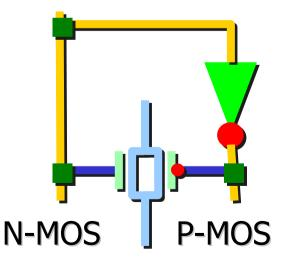
This register cell works well with a 5 V supply. In new designs ARM uses lower supply voltages where writing a `1' through the n-type pass transistor would be impossible.
