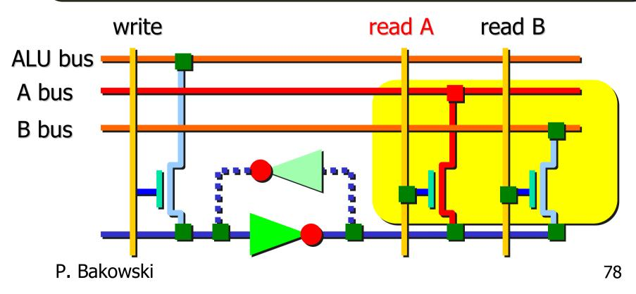
This register cell works well with a 5 V supply.
