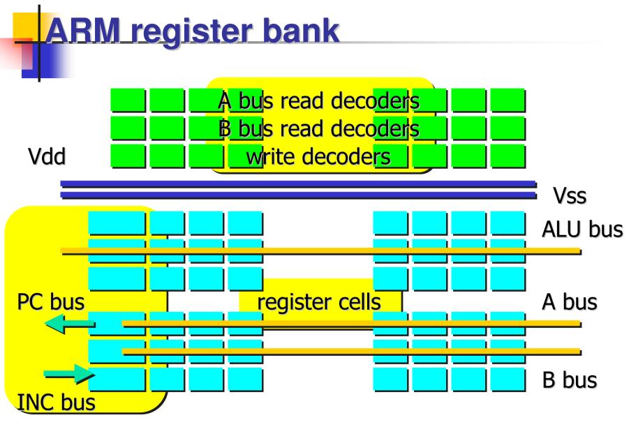
The ARM program counter register is physically part of the register bank, but it has two write and three read ports whereas the other registers have one write and two read ports.
