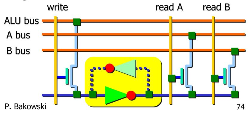
The transistor circuit of the register cell used in ARM cores up to the ARM6 is based on an asymmetric cross-coupled pair of CMOS inverters which is overdriven by a strong signal from the ALU bus when the register contents are changed.
