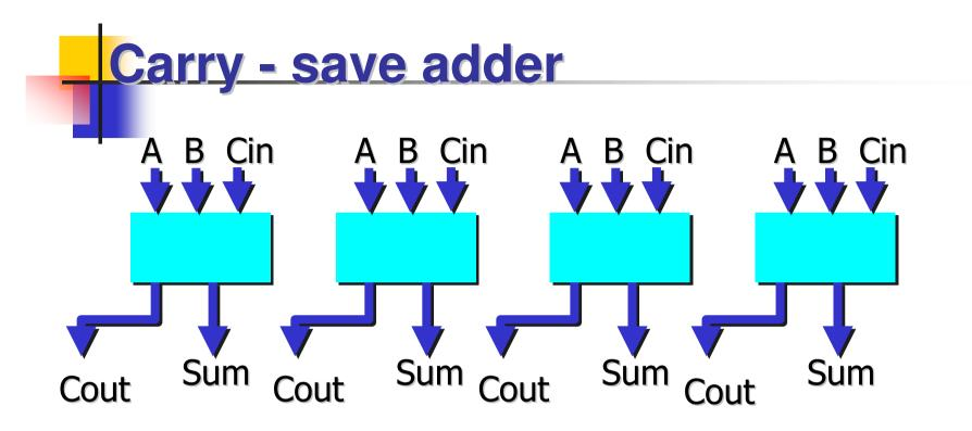
The carry-save adder takes one binary and one redundant (partial sum and partial carry) input and produces a sum in a redundant binary representation.
