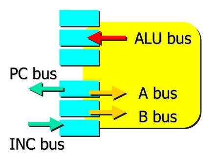
The ARM datapath is laid out to a constant pitch per bit.
