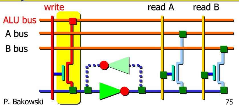
The feedback inverter is made weak in order to minimize the cell's resistance to the new value.
