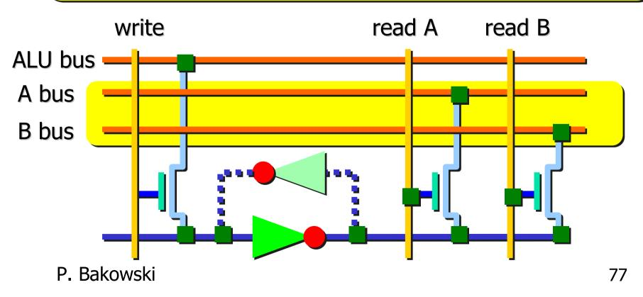
The A and B buses are pre-charged to Vdd during phase 2 of the clock cycle, so the register cell needs only discharge the read buses, which it does through n-type pass transistors when the read lines are enabled.
